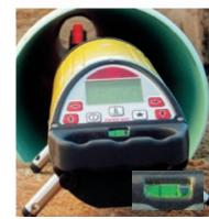
Automatic grade compensation with the housing rolled up to  $\pm$  3°, the Piper will compensate and correct for the grade errors.
